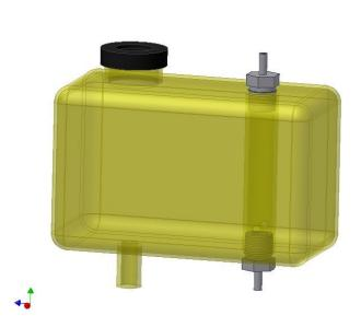
The water line has a **check valve** allowing water to flow to the HFE Cell, and a check valve in the gas line allowing gas to flow to the refill tank. I felt this necessary so that rapid gas production only flows in one direction. This should also help cool the unit, and help force bubbles off the plates.
