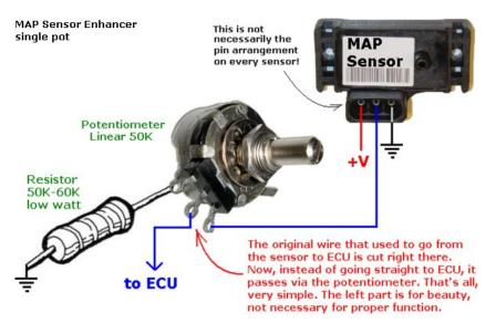
This device is totally passive and will work just the same if the signal coming in is 12 volts, 5 volts, or whatever comes on the line. The diagram here is the SIMPLEST way of doing this. The line from the sensor to the ECU is cut, and you place a pot on the line as shown. Further below you will see the improved enhancer based on the same principle.
